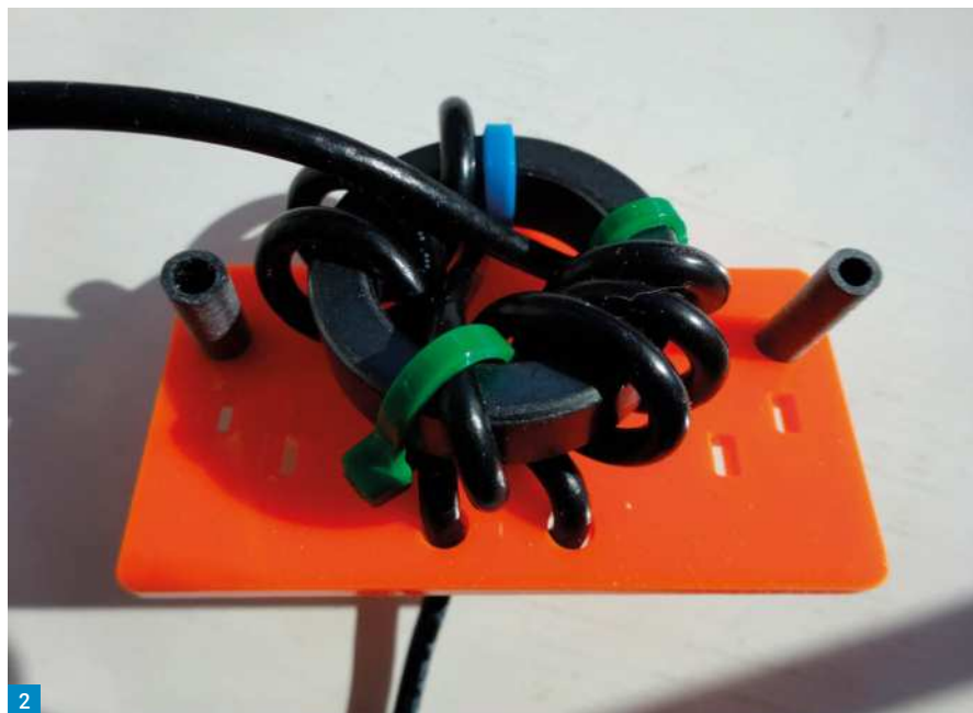
Fig. 1: A simple linked dipole covering two HF bands. When the link is open it is resonant on the higher frequency (HF1) band. When the link is closed it is resonant on the lower frequency (HF2) band. Fig. 2: The balun on one face of the centrepiece. Fig. 3: The centrepiece (opposite face to the balun). Fig. 4: A typical link before sliding the croc clip covers into place.
