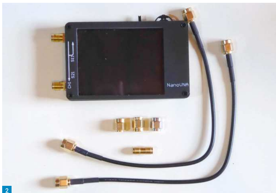
Fig. 1: NanoVNA front. Fig. 2: NanoVNA with supplied calibration standards and SMA leads (USB cable not shown). Fig. 3: Controls and the open construction. Fig. 4: Screenshot of NanoVNA-Saver software showing the six display windows.
