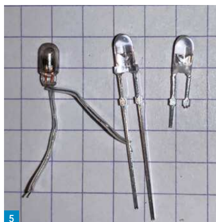
Fig. 1: The HP10525A logic probe. Fig. 2: Half shell removed. Fig. 3: Accessing the bulb. Fig. 4: LED driver circuit. Fig. 5: Comparing the bulb, an untouched LED and a cropped and filed-down LED. Fig. 6: LED with current limiting resistor and wires ready for insertion. Fig. 7: LED inserted and ready for reassembly. Fig. 8: Reassembled and ready for action.
